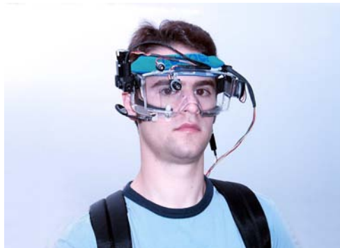
Figure 2. One of the golfers wearing an earlier version of the custom-built portable eye-tracker headgear.
