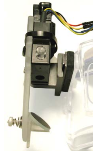
Figure 6b – Folding mirror with controlled image alignment.
