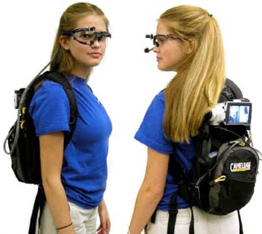
Figure 7b – Off-line eye and scene capture housed in a backpack
